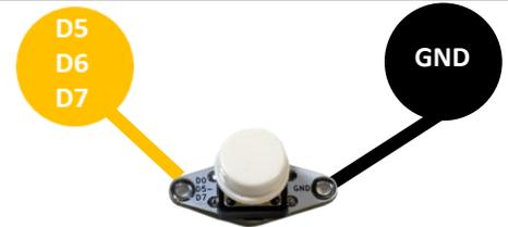
2 Check if the external button connected to D5 is pressed.
